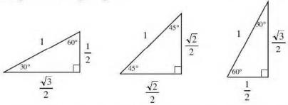
The triangles above are <u>similar</u> to the ones in the Warm-Up and illustrate the trigonometric ratios as exact values for angles of 30°, 45° and 60°.
