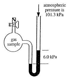
According to the diagram, the pressure of the gas in the manometer is
